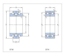
MONTON double direction angular contact thrust ball bearings are designed to locate spindle shafts in both directions. These bearings combination with cylindrical roller bearings in the NN 30 K or N 10 K series in the same housing bore. This bearing combination simplify machining of the housing bore.
